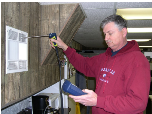
Ronnie Miller, Weatherization Auditor checks the CO Levels through a register.
